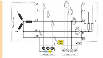
:L1 . . . . . . . . . . . . . . . . . . . . **Connection with transducers** P3 1.80 GB L2 L2 L2 L3 2 L1 ÷ PE U3 PE Tran 2 L3 1...... 600 PE Current inputs Voltage inputs
